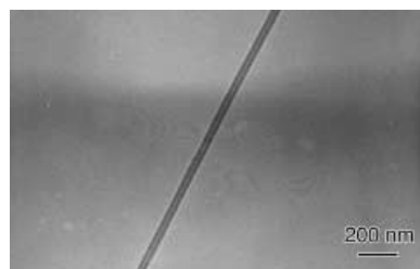
Figure 4. TEM image of a single lipid nanotube which is aligned by our manipulation method onto Formvar (poly(vinyl formal)) film spread on a copper grid.
